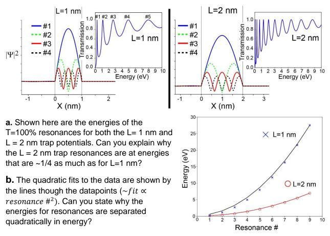
**Answer:** This is all a manifestation of particle in a box energy. **a.** The particle in a box energy is proportional to  $1/L^2$ . **b.** The particle in a box energy is proportional to quantum number squared, i.e.  $n^2$ .
