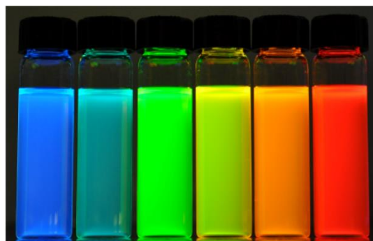
Figure 13.6. Semiconductor quantum dots change their emission color based on the size of the nanoparticle. Typical sizes are 2→10 nm.
